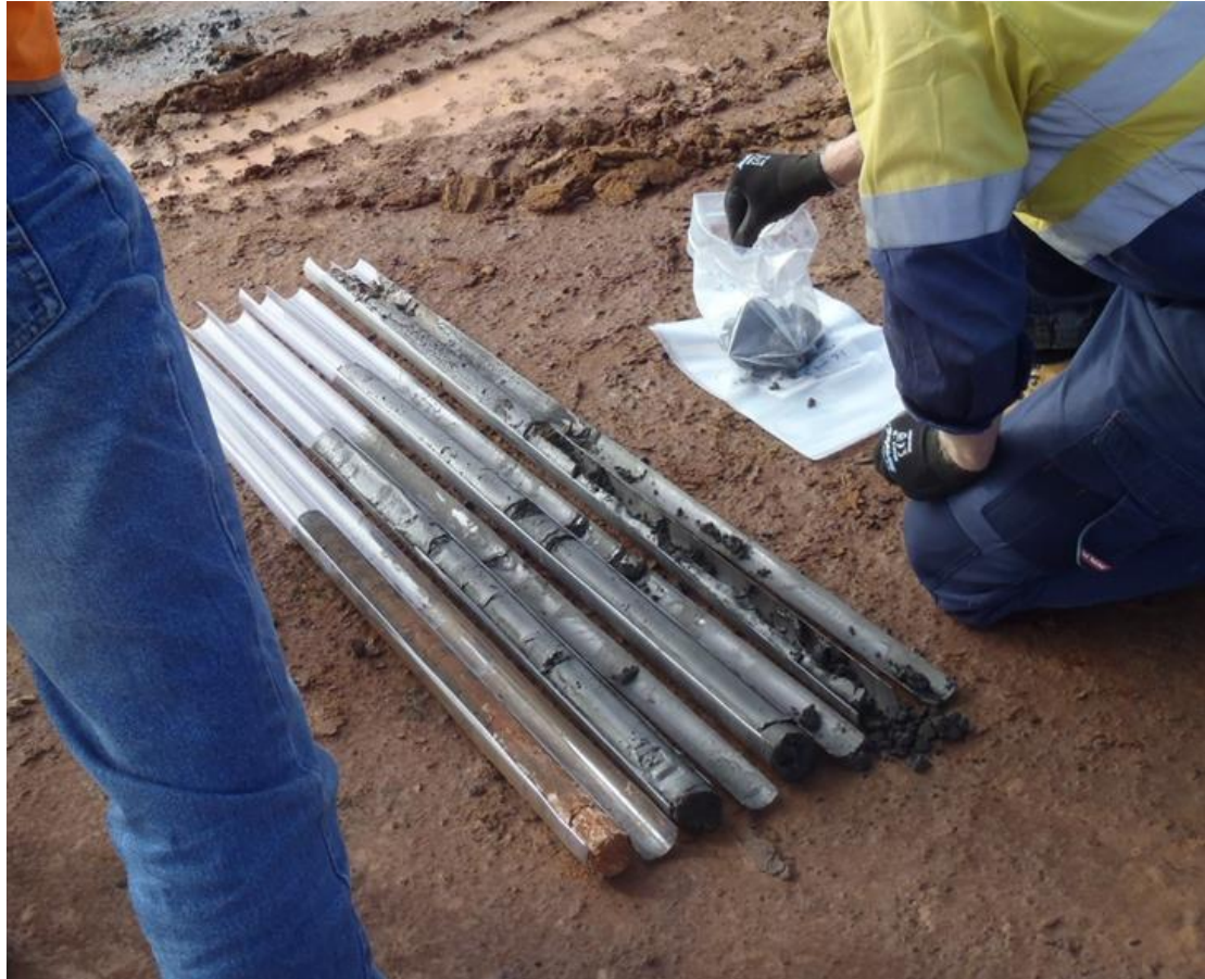
Figure 7: Push Tube Sampling
