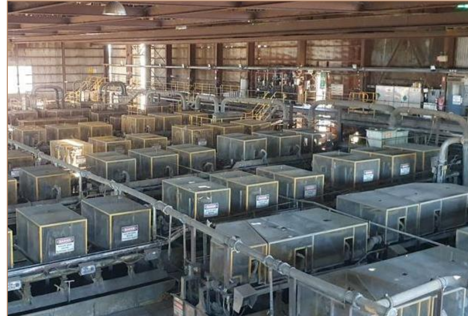
Differential Flotation Circuit
